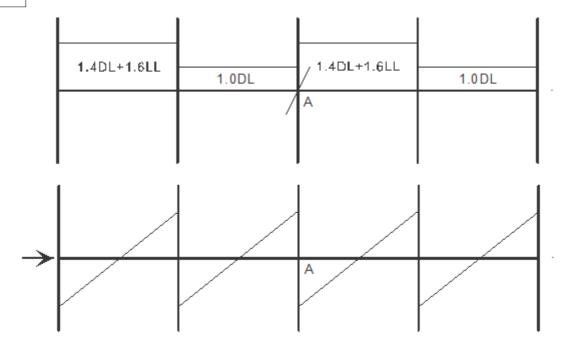
Pattern 2: Odd spans are loaded 1.0DL only and even spans are fully loaded (1.4DL+1.6LL).
