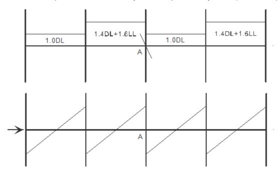
If we look at joint A, we can find the point A get the maximum rotation in anti-clockwise in pattern 1. The maximum hogging moment -Mmax, maximum sagging moment +Mmax and shear Vcol are shown as below. The same figures of pattern 2 are shown below also.
