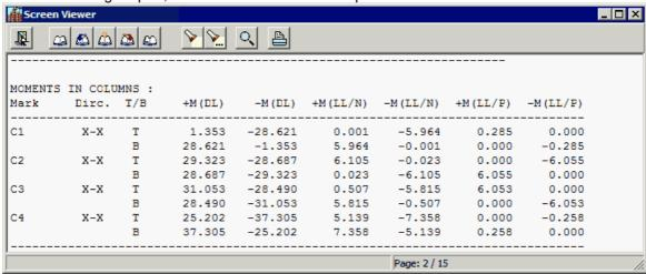
These moments are calculated from beam analysis and will be transferred to column design subcommand as design moments.
