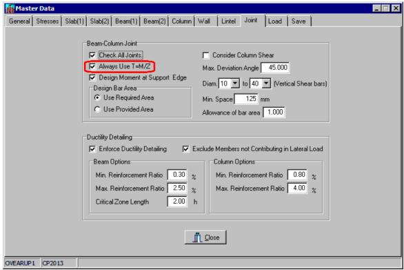
If you check this option, SADS uses T = M/z formula and ignores  $T = f_s A_{st}$  to calculate the design shear forces. You may see the value of shear force T decreased further.
