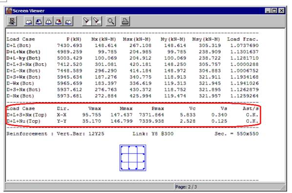
If the reinforcement is not necessary, the Ast/S is marked as O.K. otherwise the required reinforcement area is shown.
