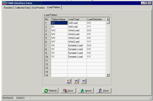
These load patterns are retrieved from Lateral Load Sub-command. You may add, insert or delete the load pattern. All load patterns you selected will be transferred to ETABS model.
