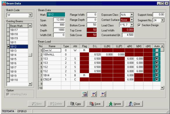
Error #1: The missing beam is 1BX5 that support on beams 1BY2 and 1BY5. SADS expects the load 1BX5 to be shown on loading list of beam 1BY2 and 1BY5. We purposely ignore these loadings for demonstrating this kind of errors. SADS can't define the location of beam 1BX5. So, the beam 1BX5 can't be shown in framing plan. You must add the missing load 1BX5 to beam 1BY2 and/or 1BY5 to fix this problem.
