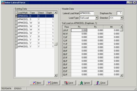
For soil loads and dynamic loads, you can calculate by hand and input to the following screen. If you use the third party application to calculate the wind loads, you should input these loads to above grid manually.
