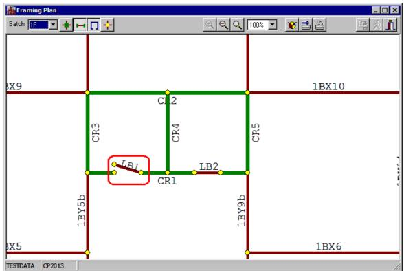
When you check the framing plan, you can find the position of LHS point of lintel LB1 is not correct. The coordinate Y of lintel LB1 should be 9.0.
