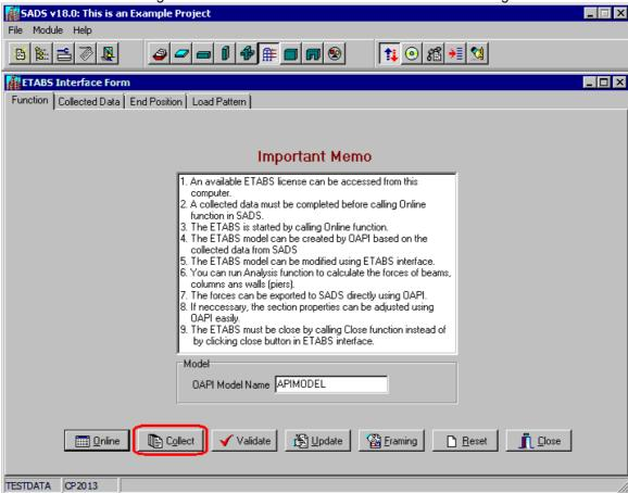
The first step is defining the OAPI model name. The default name is APIMODEL. The second is clicking the Collect button. SADS will collect the connectivity data.
