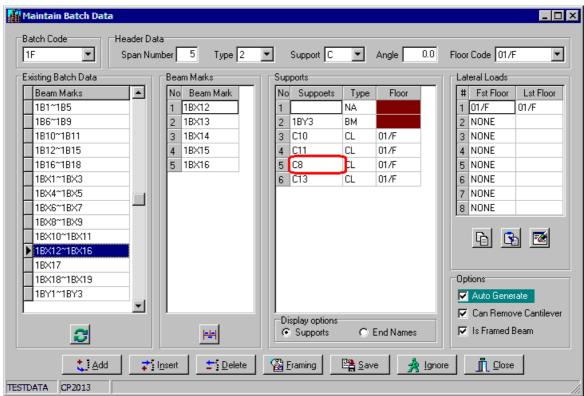
Error #2: The support #5 is C12. We mistakenly input C8 to the field. You can correct this error by inputting C12 to fix the problem.
