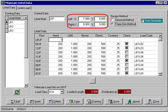
Left X and Y - the global X and Y coordinate of left end of lintel beam.
