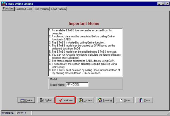
This validate is mainly validating the span and direction of beams. An example print out is shown as below.
