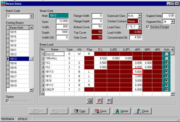
Error #3: The load position a(M) is wrong. It should be 6.0. So, the position is shifted to left. If you are using online function, the beam load that carrying framed beam, all data - name, type, attr., flag and a(M) are important. Any error in these fields may generate different problems. You may try it.
