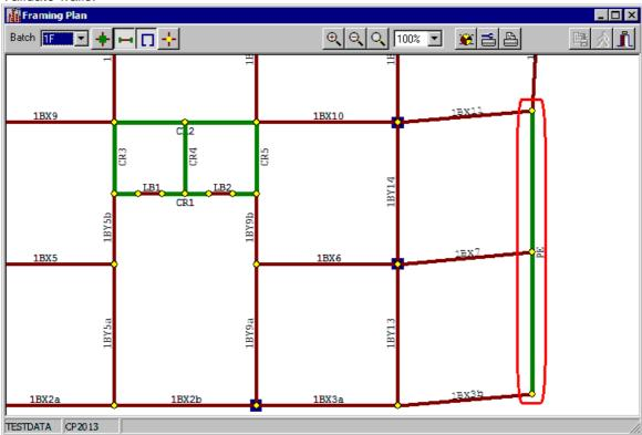
When you check this framing plan, you can find the position of wall PE is switched to up and left side. The coordinate X of wall PE should be 24.0 and Y should be 0.0..
