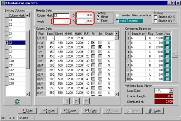
Angle - the incline angle of local X axis of column section refer to global X axis.
