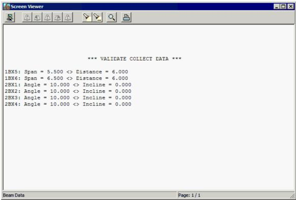
If you column and wall data has no position problem, the possible errors are caused by the errors in beam span and direction in batch data. You can fix these data errors.
