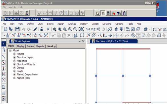
You can use SADS menu to call functions of ETABS, e.g. create new model, display existing model, run model analysis, export frame forces and pier forces, import section properties and material properties of frame members and piers, etc. Also, you can go into ETABS interface window to check the connectivity of frame object and area object, etc.
