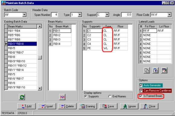
If the beam is framed beam and will be included in ETABS data, check the "Is Framed Beam" check box.
