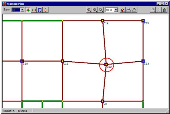
You can select the lower batch to show more columns on the framing plan. The most possible errors are the positions of columns. You can compare these positions with your paper framing plan. If you find an error, you can check the coordinates of these columns in column data window and fix the error. In this window, the coordinate X of column C12 should be 18.0 and coordinate y should 18.0 also.
