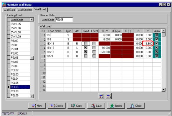
Error #4: The coordinate Y is wrong. So, the position is shifted to down. If you are using online function, the wall load that carrying framed beams, all data - load name, type, attr., X and Y are important. Any error in these fields may generate different problems. You may try it also.
